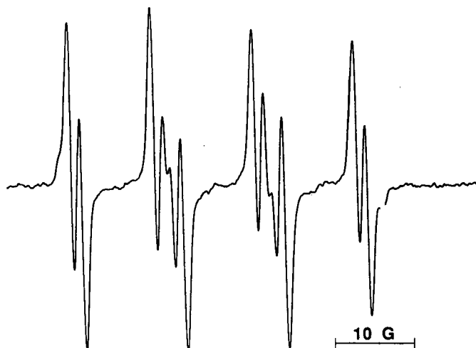
FIGURE 1 EPR spectrum of the DMPO/ O_2^- adduct in benzene. Sample was prepared by adding 20 \mu L of KO_2 stock solution to 500 \mu L of deaerated benzene containing 18-crown-6 ether (0.1 M) and DMPO (80 mM). Recording parameters: microwave power 10 mW, modulation amplitude 0.165 G, gain 1.6 \times 10^3 , scan range 100 G, time constant 0.128 G, scan time 4 min.
